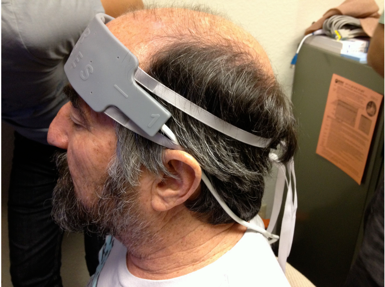
Figure 4. The fNIR device placed on the forehead of a participant. The gray flexible band contains light sources and light sensors used to infer neural activity in prefrontal cortex. Image from the GMAC Brain Imaging Lab.
