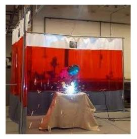
**Welding pads** – a heat-resistant fabric mat designed to protect materials underneath it against ignition; pads are placed on the surface of flammable materials directly under a hot work operation where hot debris might cause damage or start fires.
