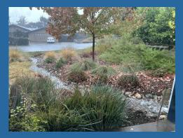
Bioswales are manmade ditches or depressions that uses plants and soil to capture, filter, and direct runoff.
